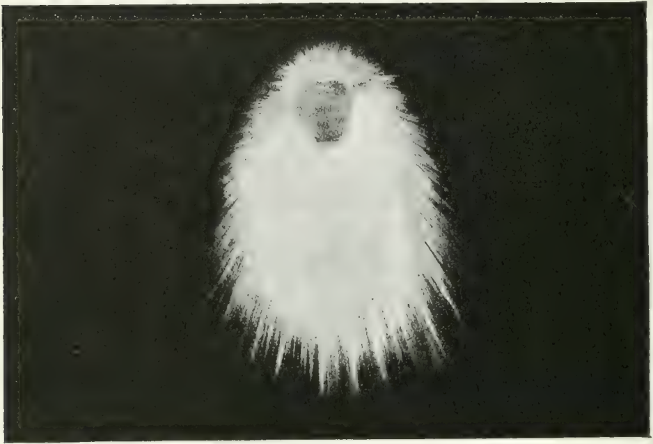
Fig. 74.—Holophane, Downward Distribution.
